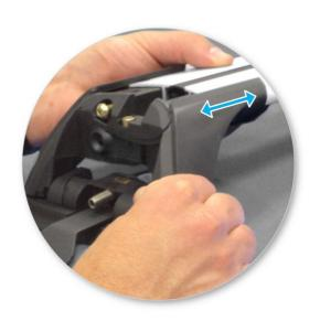
Adjust the legs on the crossbar so that they are positioned equally from the ends of the crossbar.
